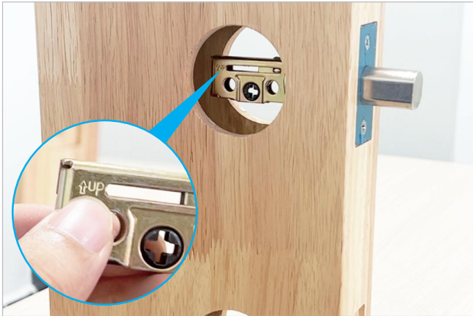
1. Adjust the length of the deadbolt D and secure it with screw M. Left open, "UP" facing indoors. Right open, "UP" facing outdoors.
