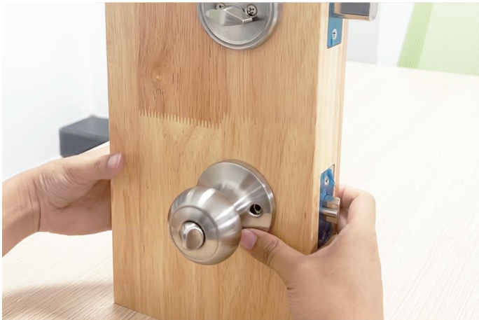
9. Install the interior parts: Ensure the interior ball knob H is centered over the positioning nut before tightening.
