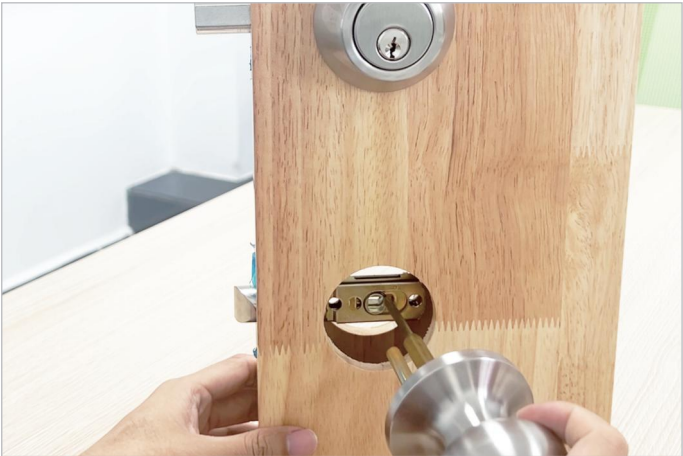
8. Install the exterior parts: Put on the ball knob G and line it up with the hole in the latch bolt.
