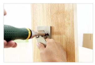
4. Install the interior parts: Secure the knob B with screw G.
